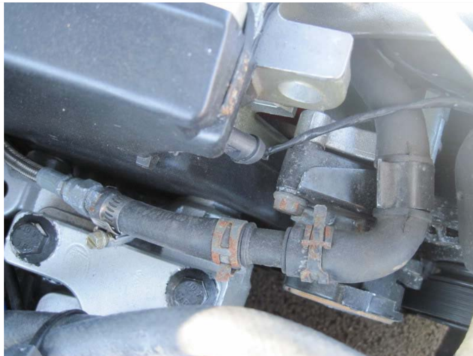
Heres another picture of where that line comes from. It comes from the coolant hard tube coming out of the block and splits between the turbo feed and coolant ball
